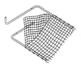
2. Weave assembled parts **A** and **C** and assembled parts **B** and **D** onto net.
