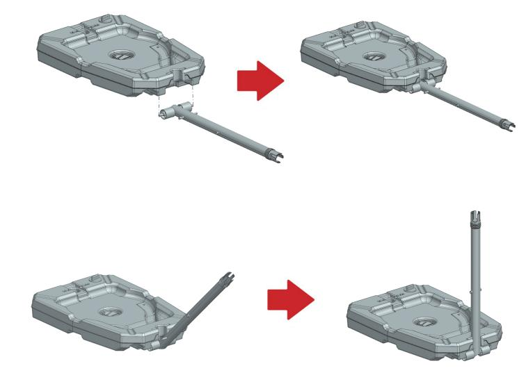
Step 3 As shown in the figure, connect the lower rod (6) and diagonal rod (5) with screws (15)
