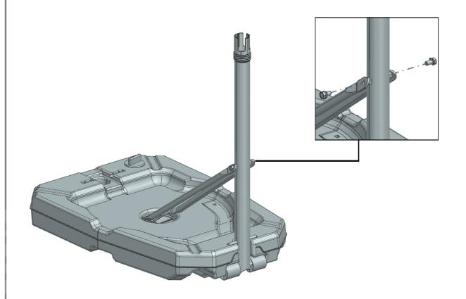
Step 4 As shown in the figure, connect the diagonal rod (5) to the base (4) with screws (14)
