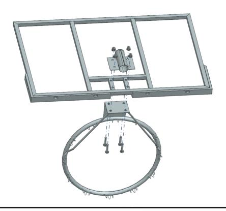
Step 6 As shown in the figure, insert the upper rod (11) into the fixing block (10) and secure it with screws (12)
