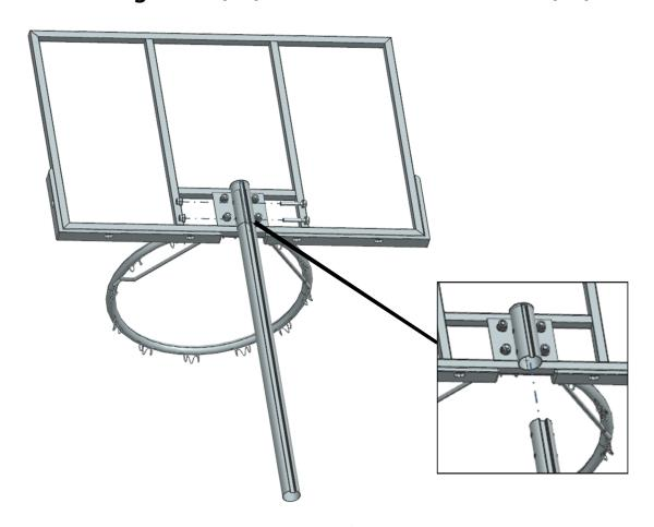
Step 7 Connect the upper rod (11), middle rod (3), and lower rod (6) together and tighten them with a knob
