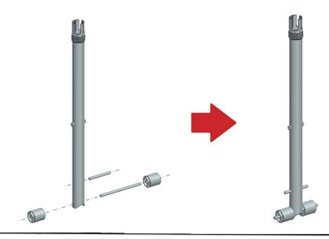
Step 2 As shown in the figure, insert the long pin (8) on the lower rod into the base (4), then rotate the lower rod 90 degrees to stand up, and finally insert the short pin (8) into the upper gap of the base (4)
