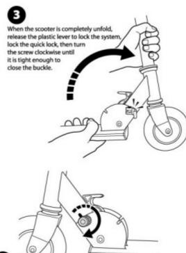
Warning! When folding the scooter, ensure that the front wheel aligned to the scooter body. If it is not done, it will not close properly. Keep fingers away from all moveable parts be the scooter as fingers could get trapped.
