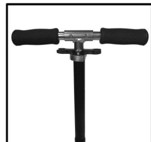
3. Release the handles from the brackets and position them in the handlebar. Make sure that the locking knob engages audibly in the preset position.
