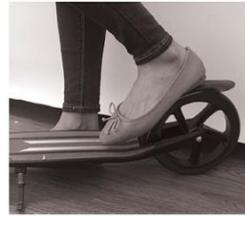
To stop faster, press the foot brake located above the rear wheel. Attention: To be used only in emergencies!
