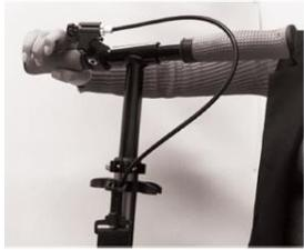
Actuate the handbrake lever by pulling the lever in your direction. The handbrake reduces the speed without coming to a sudden stop.
