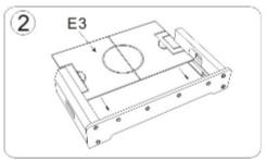
Insert the bottom board into the assembled boards of 1step.
