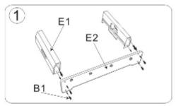
Assemble two short boards and one long board, then connected by screws.
