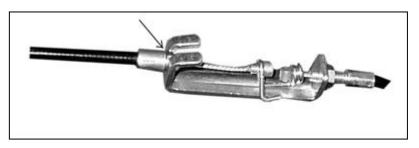
Drop down the Connector so the fitting sits firmly on top of the bracket.
