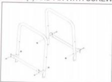
STEP 4: SELECT PART (2) AND PART (1) TO ASSEMBLE. PART (2) HAS RUBBER TUBING PROTECTING IT. PLEASE NOTE PART (2) DOUBLE-HEADED.
