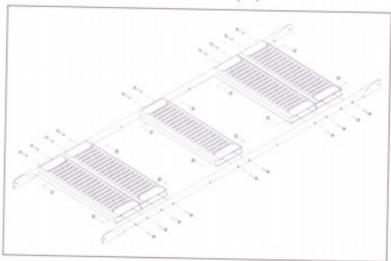
STEP 3: SELECT PART (3) AND PART (4) AND FIX WITH SCREW (8) AND NUT (11).
