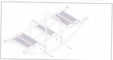
STEP 6: THE REMAINING PART (6) MUST BE ASSEMBLED FIRST WITH PART (1) AND THEN WITH PART (2). WHEN FINISHED, MAKE SURE ALL SCREWS ARE TIGHT.
