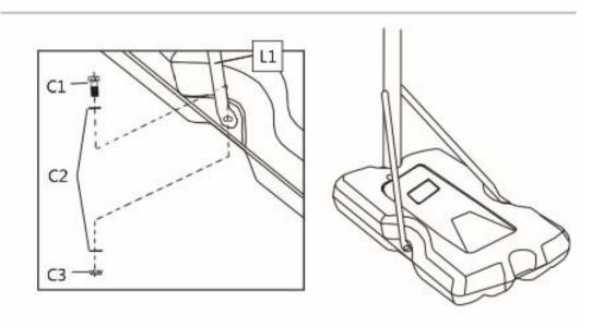
Fix the other end of Pole Brace(L1)&(L2) on two sides of Base(S) by Bolt Set (C1), (C2)&(C3) as shown.
