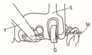
Insert the Wheel Shaft (M) into Wheel(G),Base(S) and end of Bottom Pole (Y) as shown.
