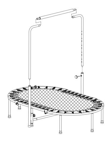
6. Stand on the trampoline to ensure legs and handrails is leveled and sturdy. Install and tighten adjustment knobs (7) and two small knobs (12)to lock the handrail supports (8) in position.
