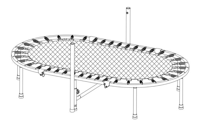
5. Insert the middle handrail (10)into the right(9)and left handrails(9), and lock with the button pins . Insert the left and Right handrails into the handrails support (8) and lock in position with the two adjustment knobs(7).
