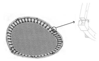
Warning: do not allow your fingers to touch the end of the panels in the hinge-joint areas while you are folding or unfolding the trampoline. If your gingers get caught between the ends of the panels, pinching can cause serious injuries !
