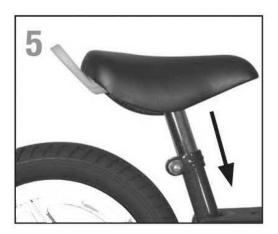
Stick the saddle into the seat post. Take note of the marker on the seat post indicating the minimum depth it should be stuck in. Adjust the saddle to the centre and tighten the clamp.
