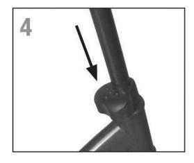
4. Push the covering cap over the handlebar clamp.
