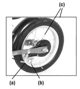
After each adjustment, check that the wheel can move freely as otherwise the brakes could get damaged.
