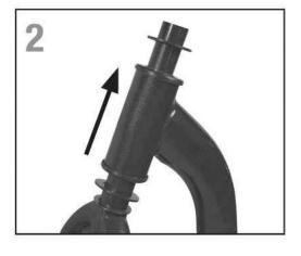
Push the fork from below through the frame, as shown in the diagram. Make sure there is a plastic ring above and below the frame.
