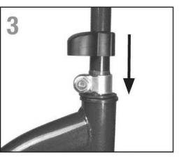
3. Push the covering cap over the handlebar rod.
